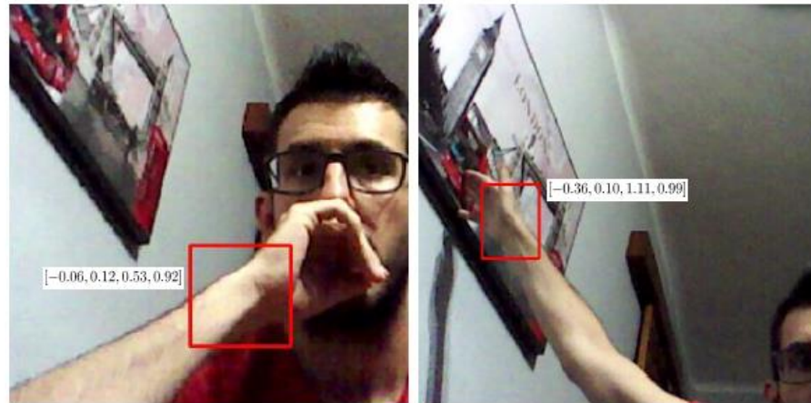
Fig. 8. Localization of the wrist in two different positions, showing the pose obtained with respect to the reference system of the camera and the class score in the detection vector [x, y, z, \mathcal{L}] . Note that in both pictures \mathcal{L} > 90\% .
