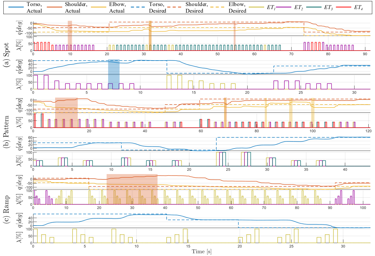
Fig. 5: Excerpt of data from one particular subject collected during the modality experiment. For the three feedback modalities (a) Spot, (b) Pattern, and (c) Ramp, each subplot represents the variation of the actual (solid line) and desired angles (dashed line) of the arm (top) and torso (bottom) joints. The subplot at the bottom of each row provides the amplitude of vibration ( \lambda ) of each ErgoTac device. Note that only four ErgoTac devices ( ET_{1,\dots,4} ) were used simultaneously in this set of experiments, as the arm and torso tests were carried out separately. The semi-transparent red, yellow and blue areas determine when the subject misunderstood the feedback and moved in a wrong direction the shoulder, elbow or torso, respectively.
