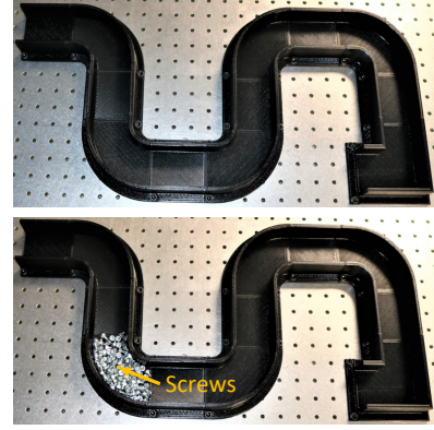
Fig. 5. Experimental setup: (top) is the maze path for the first experiment. (bottom) is the maze with a cluttered condition by screws for the second experiment.
