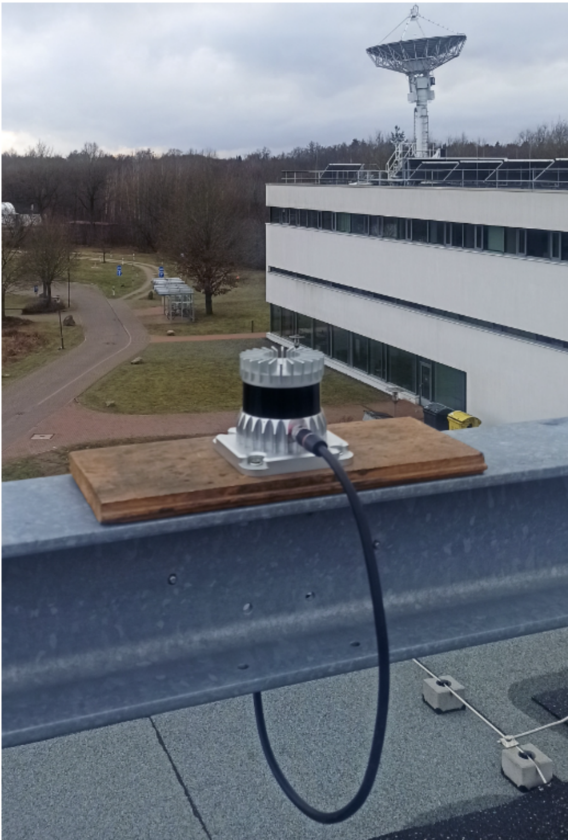
Figure B.2: Configuration and positioning of the Ouster sensor for the validation campaign.
