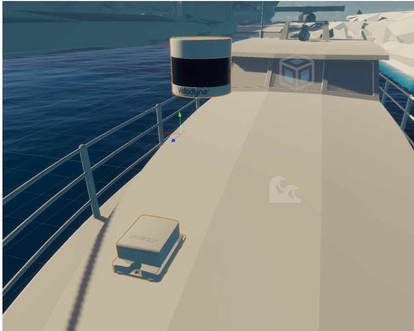
Figure 3.12: IMU and LiDAR sensors integrated into Unity. The sensors are positioned relative to the AURORA vessel's structure, ensuring accurate alignment with the ship's coordinate system. Their placement is designed to be easily adjustable, allowing for repositioning to different locations on the vessel. This flexibility enables testing various configurations and scenarios, enhancing the versatility of the simulation environment.
